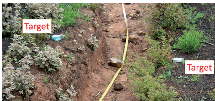
Fig. 2 - Positioning of the targets in the edges of the trail to work with common spatial points in the photos.
